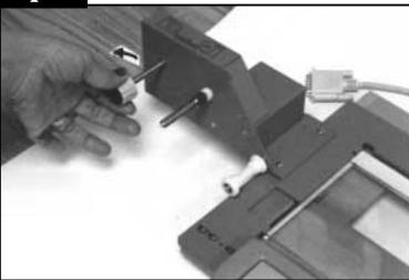
The Carrier has two manual knobs which are used to manually advance or rewind the film.
